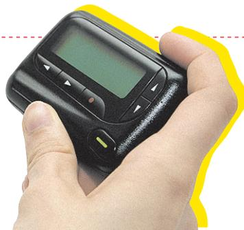
**...THE PAGER SENDS TEXT MESSAGES THROUGH THE RADIO?** The user has to call an operator and tell the message to a person who types it up and then sends it through the radio to the receiver's device.
